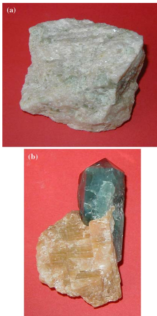
Fig. 1 Polycrystalline (a) and single-crystalline (b) FA of geological origin. The single crystal has a grey-green color due to incorporated transition metals
